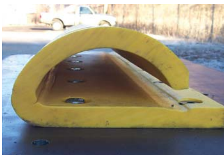
Ultra Poly's FLEXI FEND® high impact UHMW fender system prior to impact test.
