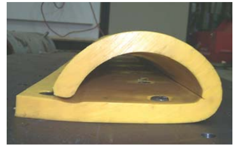
FLEXI FEND® after 2,000-pound impact test. The unique leaf spring shape of FLEXI FEND® allows it to flex with impact and return to shape. Fenders fully recover from repeated collisions and heavy loads.
